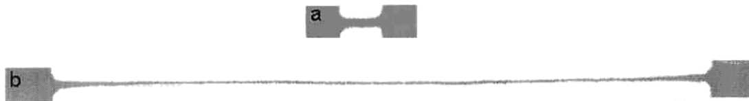
FIGURE 3. Sample of Zn-22% Al alloy before (a) and after (b) testing under superplasticity conditions
